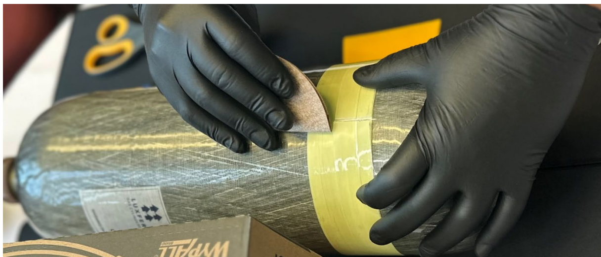
Figure 3: Abrading the surface over the delamination
