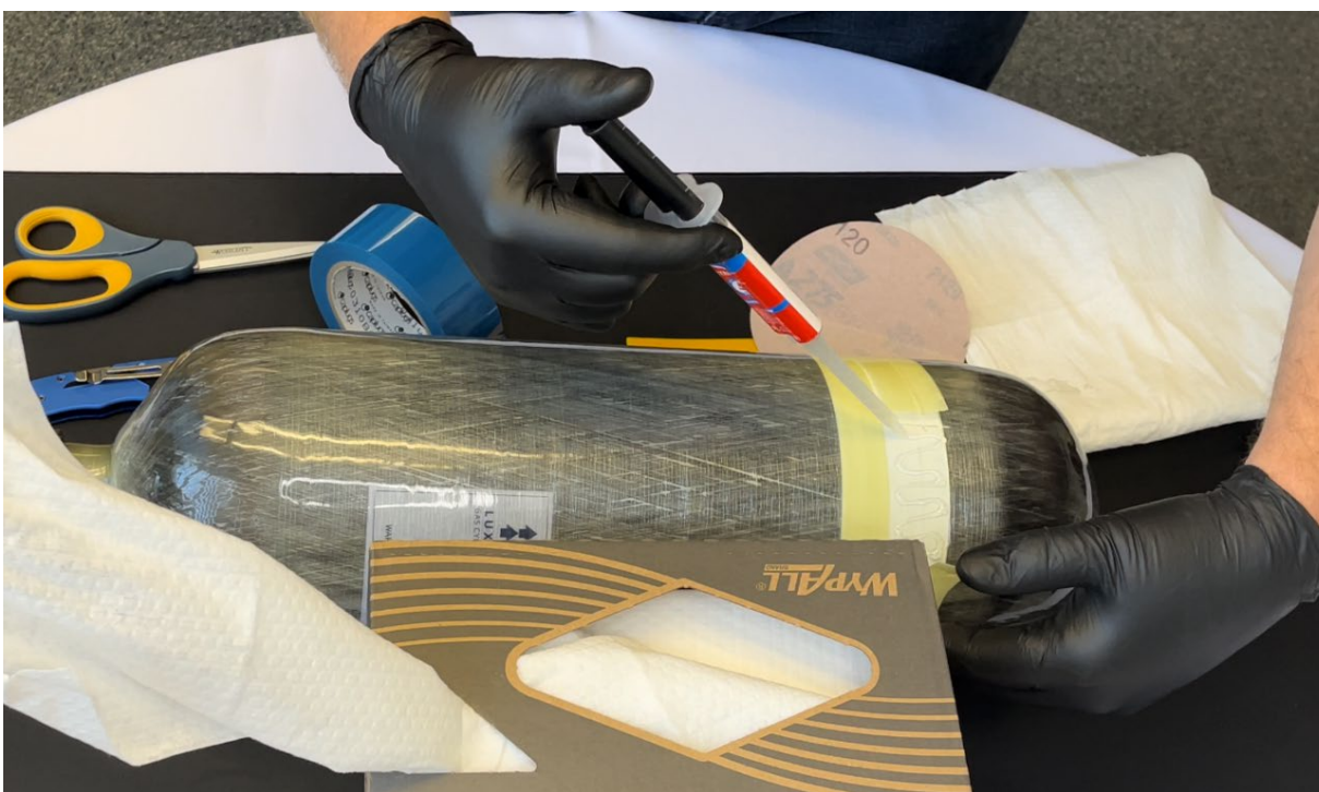
Figure 4: Application of two-part 5-minute epoxy under delamination
