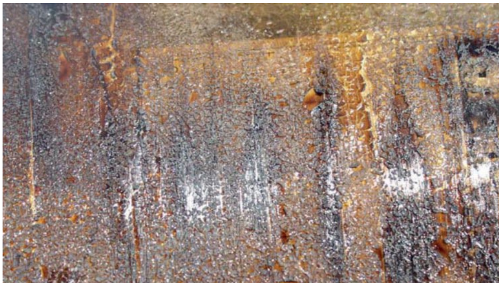
Level 3 damage like this required the cylinder to be rejected.
