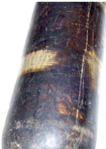
This smoke-darkened cylinder only has Level 1 damage. After cleaning, it can be returned to service.
