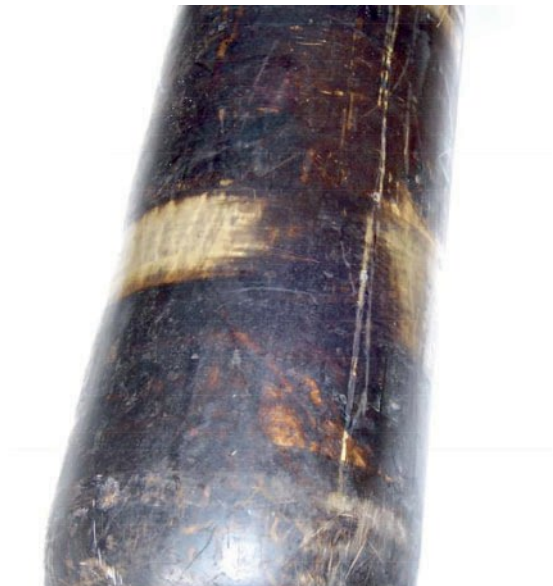
This smoke-darkened cylinder only has Level 1 damage. After cleaning, it can be returned to service.
