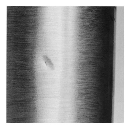
**PHOTO 1.** Dented cylinder. This cylinder has a 'brushed finish' with a clear coating.
