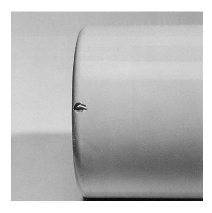
**PHOTO 3.** Cylinder shows signs of having been in an accident or dropped. May have been struck or fallen. The inspector, seeing an obvious deviation on an otherwise uniform cylinder should ask the owner if he/she is aware of any cause for such a mark.
