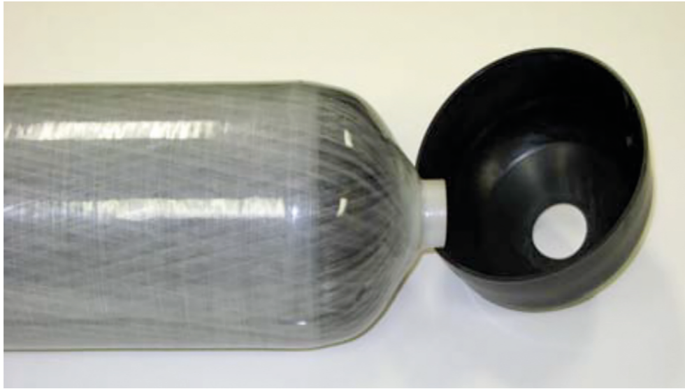
Cylinder surface after cap has been removed.
