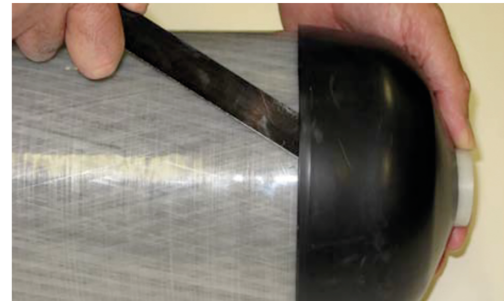
Note the depth of the blade under the cap. The adhesive head is 20-30mm from the edge.
