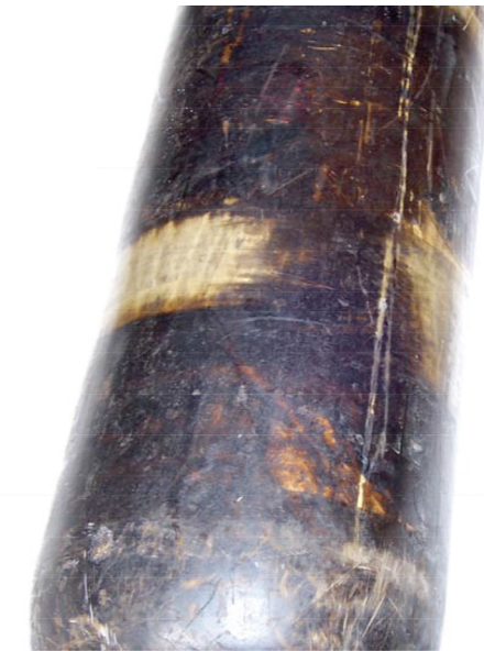
This smoke-darkened cylinder only has Level 1 damage. After cleaning, it can be returned to service.
