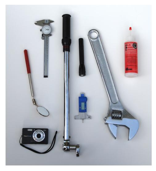
A mirror and a flashlight are helpful when you are inspecting hard-to-reach areas. Bubbling leak-detection fluid is also useful. (*Optional:* A digital camera can be used to document damaged areas.) Fill out an inspection report form (available from Luxfer.) If a cylinder is irreparably damaged, apply a "Danger: Failed Cylinder Inspection" label to cylinder. If the cylinder passes inspection, apply a label showing the date of the inspection.
