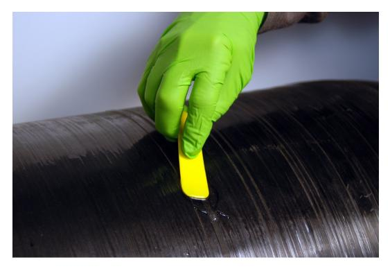
▲ Follow the procedures shown previously above to mix epoxy resin. Generously apply resin to the gap left when delaminated fiber was removed from the outer hoop-wrapping.
