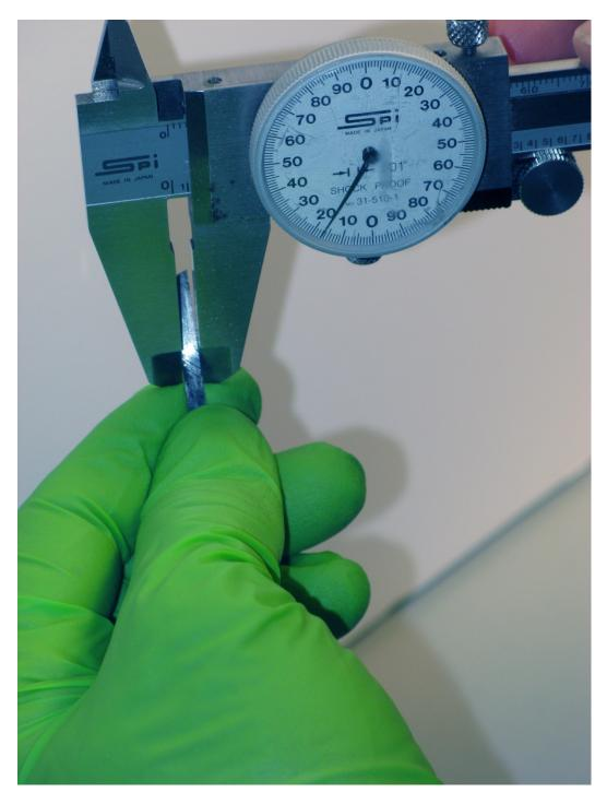
▲ Measure the width of the clipped segment to make sure that the delaminated area is within acceptable limits for repair.
