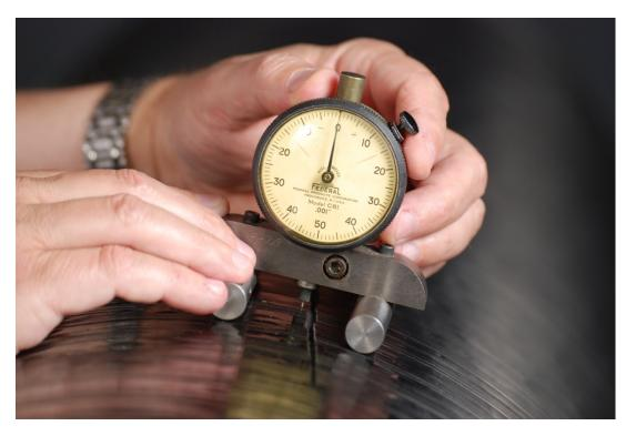
▲ **Cut measurement**—First calibrate the depth gauge to zero on the undamaged cylinder surface.
