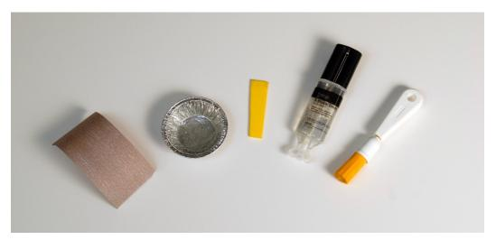
These tools are needed to repair Level 2 damage (left to right): 120-grit (fine) sandpaper, a receptacle for mixing epoxy resin, a resin applicator, two-part epoxy resin (resin plus cure) and a brush that may be needed for removing dust and debris. Clean shop rags or heavy-duty paper towels are also useful.
