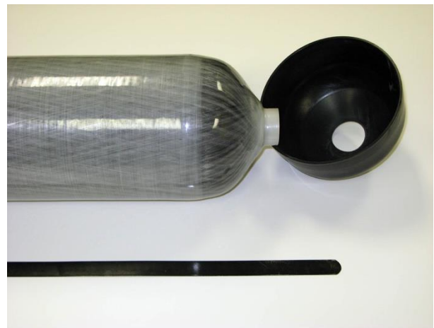
Photo 2: Cylinder surface after cap has been removed.
