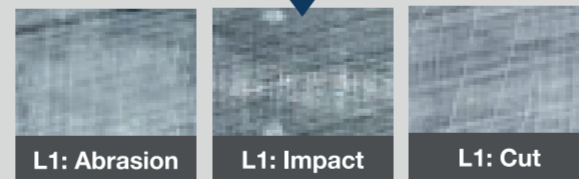
LEVEL 1 – MINOR Continue with fill - see valves.
