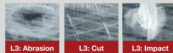
LEVEL 3 – MAJOR CONDEMNED Cylinder must be condemned and removed from service. See section 6 of the Luxfer LCX User Manual for more information on damage levels and methods of repair.
